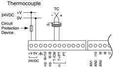
Thermocouple 0: use T- Input as negative input and T+ as positive.
